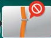
Do **NOT** run through walls, doorways, ceilings or floors. If cord is covered, heat cannot escape, which may result in a **FIRE HAZARD**.
